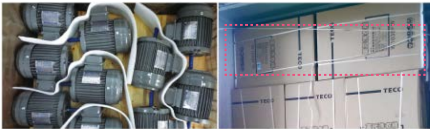
Photo: Domestically sold motors are shipped in mesh cage with minimal protective packaging. Photo: Washing machine packaging is designed to facilitate flat packing, increasing transport capacity by 28% (increasing container capacity from 136 units to 174 units)
