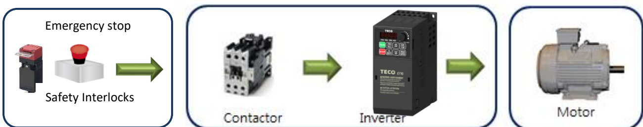
Electromechanical. Without STO function SIL 2. Stop Category 0
