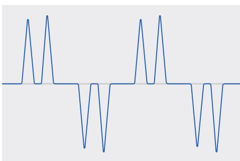
Before using F510 Harmonics not improved THDi \geq 100%
