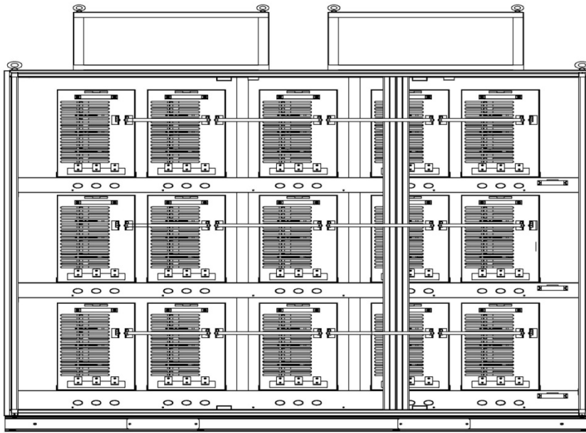
Figure 3-16 Diagram of Wiring Terminals inside Transformer Cabinet
