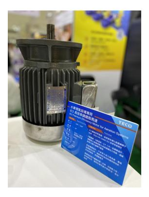
The "nine-furrow motor" is designed for application in oxygenenhancement equipment of waterwheel, boasting long product life, at least three years longer than existing model, thanks to use of key stainless-steel components with high anti-corrosion and weather-endurance capabilities. Due to high electricity efficiency, installation cost can be recouped within half a year to one year.
