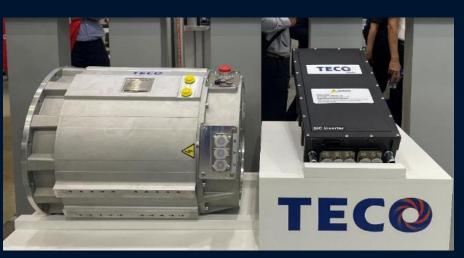
TECO unveiled self-developed SiC High Efficiency Drive, features SiC modular direct drive, skipping gear reducer and thus avoiding attrition, which results in ultra-high efficiency and higher power density. With a compact case, only half the size of common model, the product is applicable to 12 meter-long e-bus, inter-city e-shuttle bus, large e-truck, and engineering machinery.
